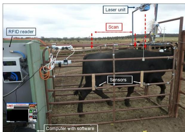
Figure 2. Stationary laser setup showing positioning of laser unit, activating sensors and associated equipment
