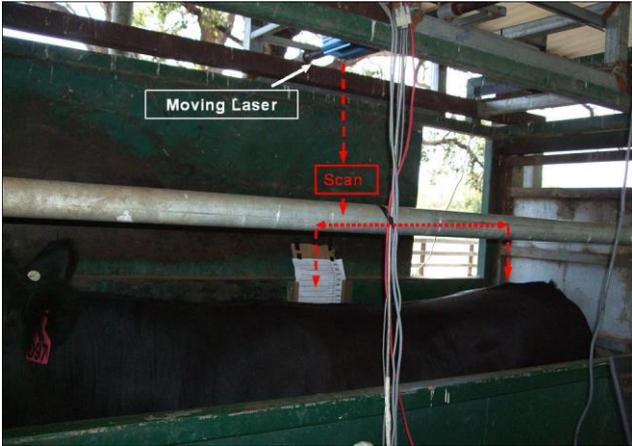
Figure 3. Moving laser setup showing positioning of laser unit on the movable carriage
